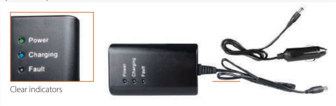
TR8180 DC Vehicle Charger Charge from your Vehicle to 12V LiFePO 4 Tracer have developed a DC to DC charger with a 'Buck Booster' circuit. (1m lead) This charger enables the *LiFePO 4 battery to be charged from a vehicle 12V socket. The input voltage to the buck booster can be from 9-16V DC and the output voltage is stabilised at 14V, the voltage needed to charge a LiFePO 4 battery. Maximum output current is 2A.
