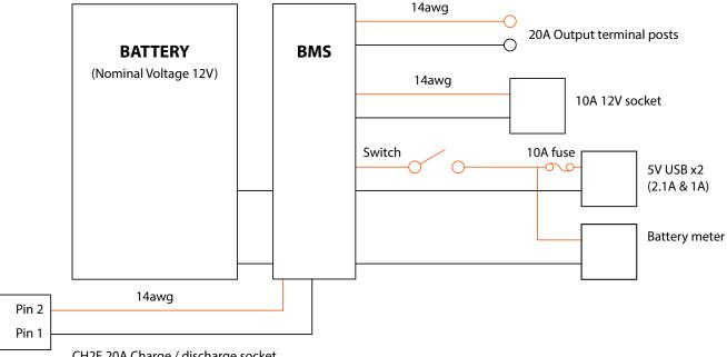
CH2F 20A Charge / discharge socket
